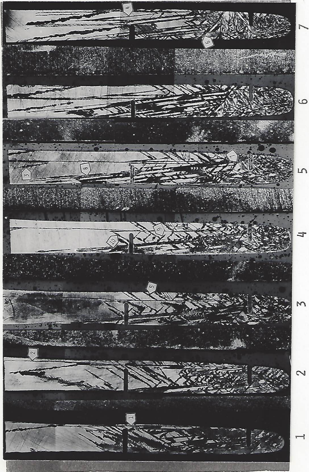
0.045 0.16 0.04 0.105 0.10 0.07 AMOUNT REMOVED (MM) FIG. 15 METALLOGRAPHIC PANORAMAS OF SPECIMEN F (ALLOY 2) (12.2X)
