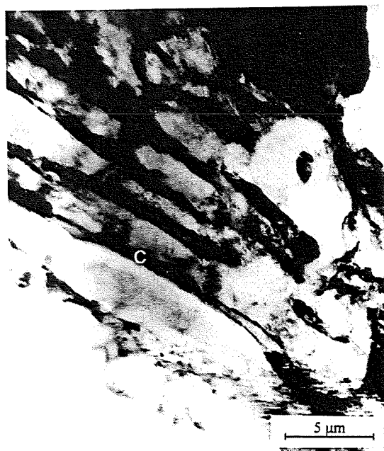
Figs. 8.18 (above) and 8.19 (below): Micrographs of pearlite in steel H271 (Fe-0.25C-0.9Mn-1.7Si). STEM of undeformed and TEM of deformed respectively, showing cementite diffraction pattern of point C and dark field image using 04\bar{2} spot.
