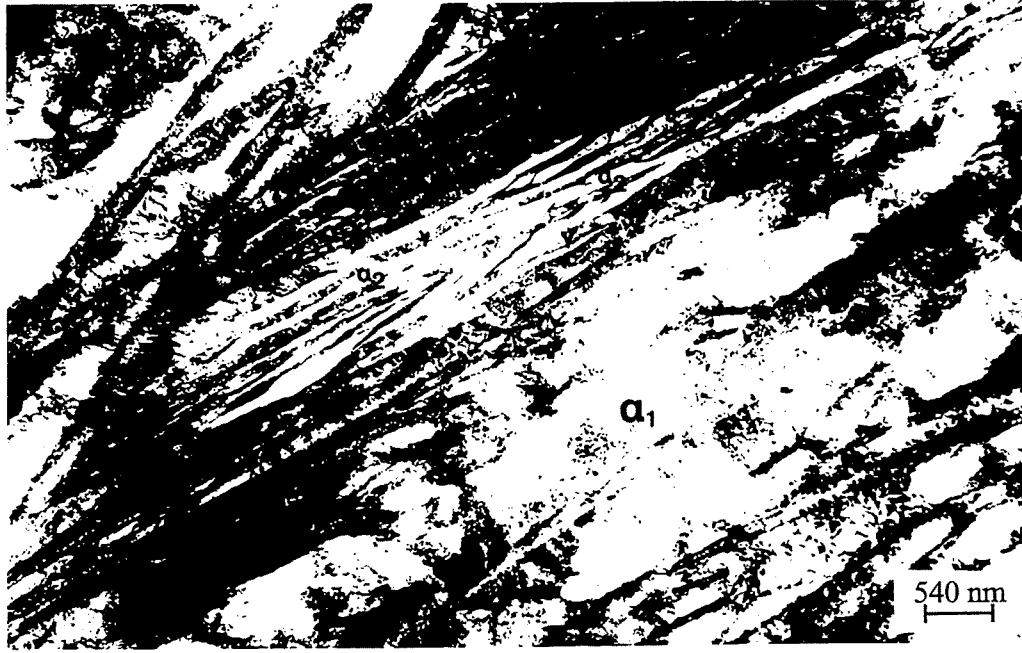
Fig. 4.9: TEM micrograph of bainite sub-units of two different widths corresponding to transformation ( \alpha_1 ) at 420°C for 30 minutes and then ( \alpha_2 ) at 290 °C for 21 days for steel Fe-0.9C-3.9Si wt.% [Papadimitriou and Fourlaris, 1997].
