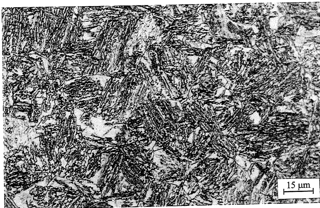
Fig. 4.20: Optical micrograph of continuous cooling sample of Fe-0.38C-1.29Si-1.73Mn wt.% steel with cooling rate 0.1\text{ }^{\circ}\text{C s}^{-1} from 450\text{ }^{\circ}\text{C} to 250\text{ }^{\circ}\text{C} . Etched with 2% Nital to show the bainitic microstructure.
