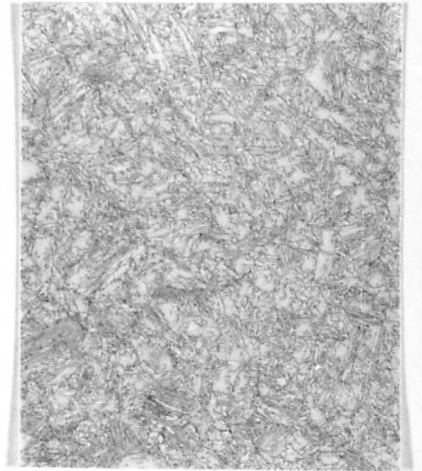
Fig. 3.1: Optical micrographs for alloy C reacted across the bainite formation range.
