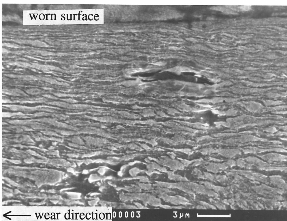
Fig. 8.19: SEM micrographs of a MnS inclusion situated near the worn surface has been flattened , but no crack can be observed, after wear test. Alloy K2, Fe-0.49C-1.53Si-2.03Mn (wt.%), 900 °C @ 1800 s → 355 °C @ 7200 s → water quenched.
