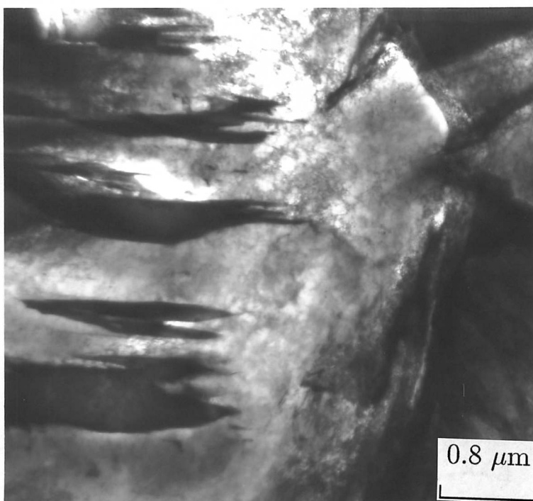
Fig. 8.7: TEM bright-field micrograph shows carbide free upper bainite grew from grain boundary ferrite. Alloy P1, Fe-0.49C-1.44Si-0.51Mn-3.5Ni (wt.%), 900 °C @ 1800 s → 370 °C @ 3600 s → water quenched.
