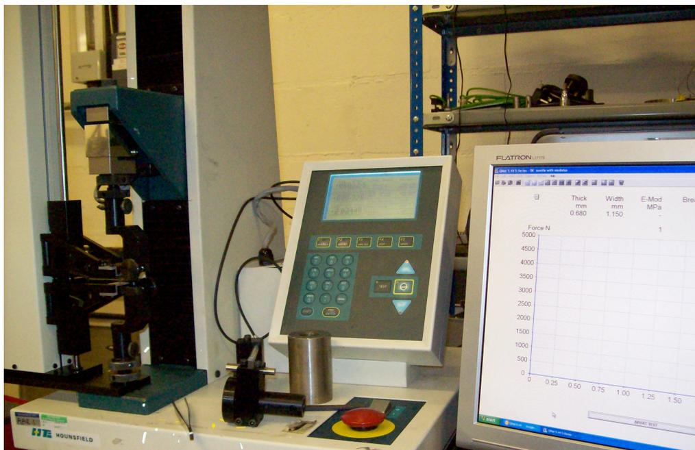
**Figure 3.7: Hounsfield Low Load Electric Screw Machine, maximum load 5 kN [65].**
