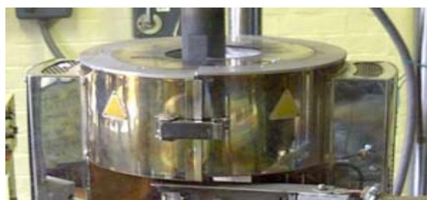
**Figure 3.5: LCF testing machine with a maximum load of 100 kN plane strain fracture toughness test [64].**
