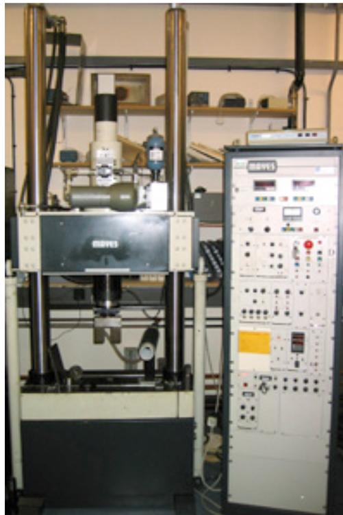
**Figure 3.4: Mayes 100 kN servo hydraulic axial fatigue testing machine [63].**
