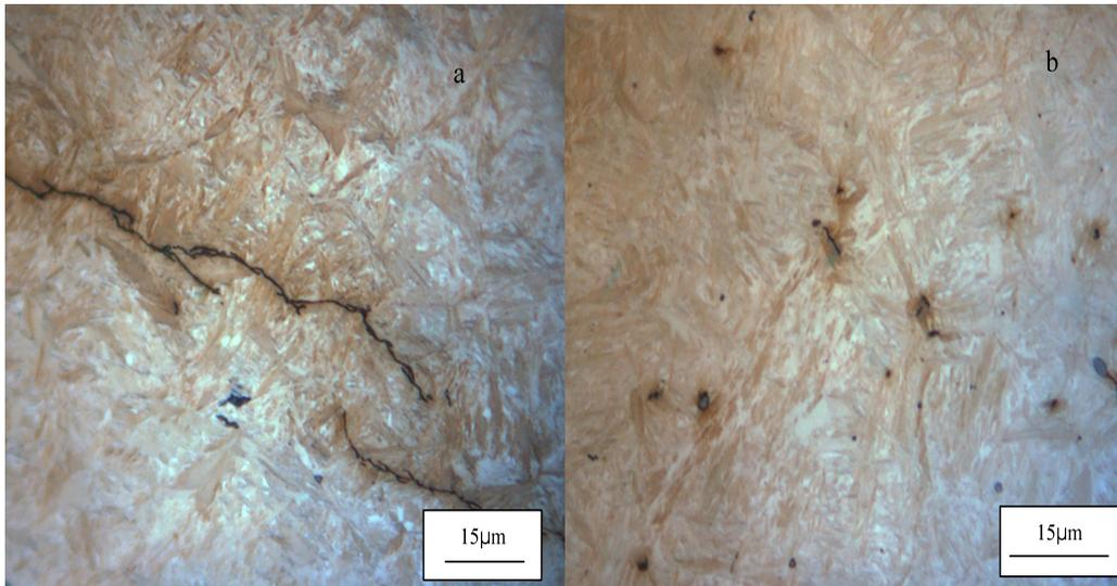
**Figure 7.8: Extent of micro-cracking in alloy EE25 after direct quenching from the austenitisation temperature of (a) 930 °C, (b) 800 °C.**
