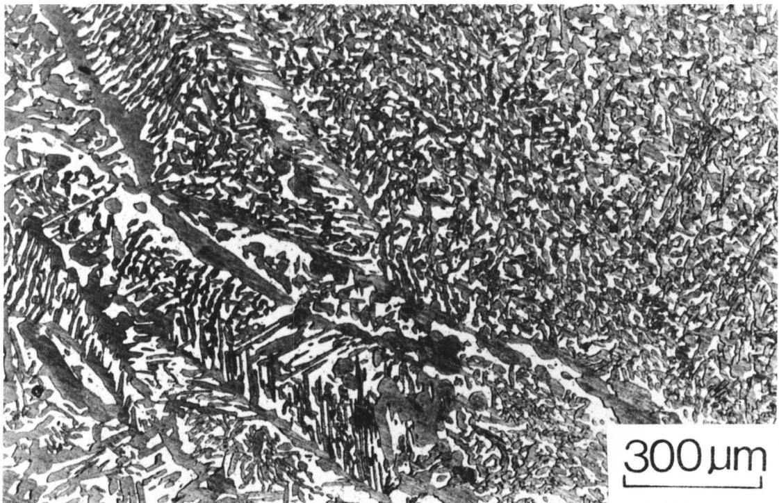
Fig. 7.7.c: Microstructure of welded alloy WR4 after ageing at 1120°C for eight days. The dark etching phase is austenite and the measured hardness of the specimen is (VHN 223).
