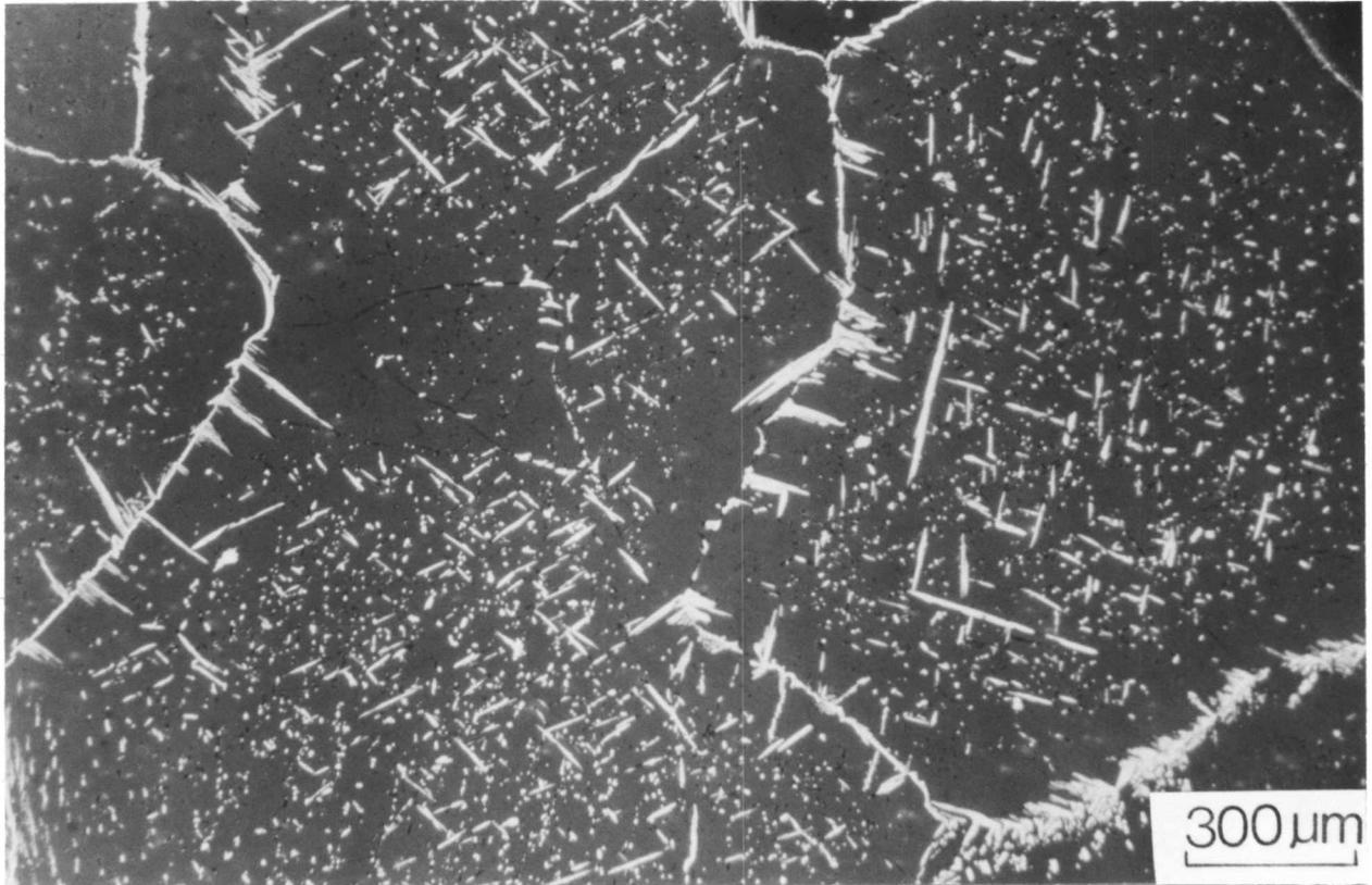
Fig. 8.2: Microstructure of a deformed SH specimen after continuous cooling treatment ( $Q = 0.11^{\circ}\text{C s}^{-1}$ ). The light etching phase is austenite.
