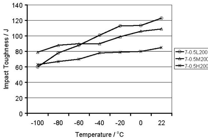
**Figure 3** Impact toughness plots that show the effect of increasing carbon from 0.03 to 0.11 wt. % at 7Ni and 0.5 Mn.
