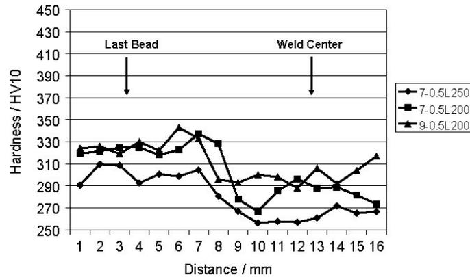
**Figure 5** Hardness plots showing the effect of increasing Ni from 7 to 9 wt. % with Mn levels 0.5 wt. %. Also shown is the effect of reducing interpass temperature at a Mn content of 0.5 wt. %.
