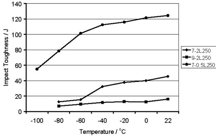
**Figure 1** Charpy impact toughness plots showing the effect of increasing Ni from 7 to 9 wt. % and the effect of reducing Mn from 2 to 0.5 wt. %.
