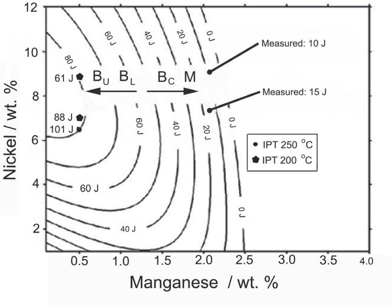
**Figure 7** Comparison between recorded and predicted impact toughness at -60 °C as a function of manganese and nickel content. See Part A [22] for details of the modelling. Upper bainite is B<sub>U</sub>, lower bainite is B<sub>L</sub>, coalesced bainite is B<sub>C</sub> and martensite is M. These were the observed microstructures from microstructural investigations.
