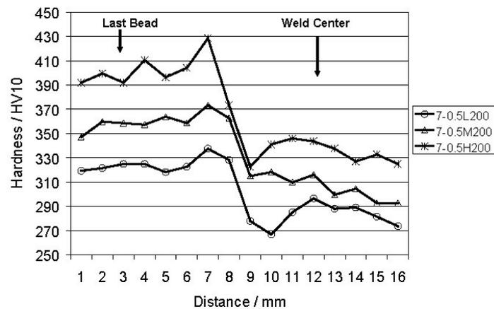
**Figure 6** The effect on hardness of increasing C from 0.03 to 0.11 wt %
