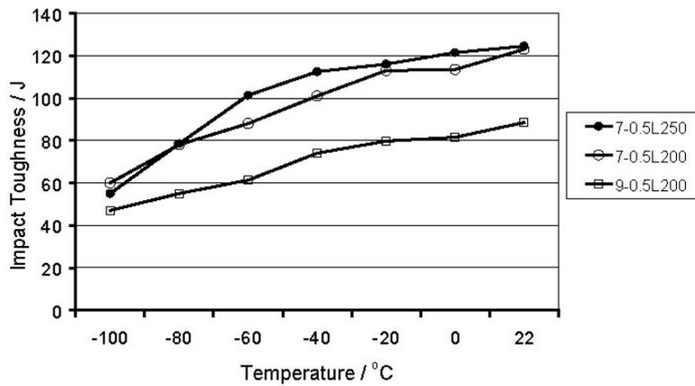
**Figure 2** Impact toughness plots illustrating the effect of increasing Ni from 7 to 9 wt. % with Mn level at 0.5 wt. %. Also shown is the effect of increasing interpass temperature for the 7 Ni weld metals.
