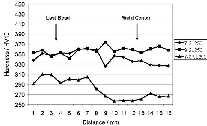
**Figure 4** A comparison of hardness measurements that show the effect of increasing Ni from 7 to 9 wt. % and the effect of reducing Mn from 2 to 0.5 wt. % at 7 wt. % Ni.
