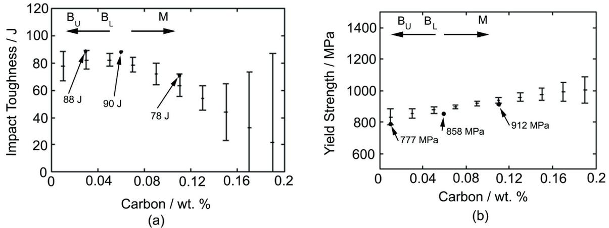
**Figure 8** A comparison between the recorded impact toughness at  $-60^{\circ}\text{C}$  (a) along with yield strength (b) versus the neural network predictions as a function of carbon content for 7 wt. % Ni combined with 0.5 wt. % Mn. Also shown are the microstructural changes in relation to the increasing carbon content as was observed with microstructural investigations.  $B_U$  is upper bainite,  $B_L$  is lower bainite and M is martensite.
