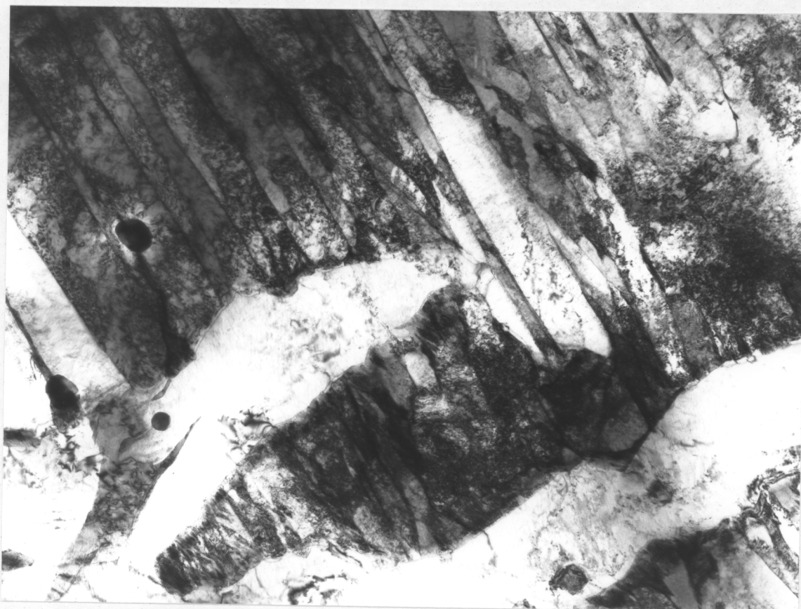
Figure IV.6(e) - Reaustenitisation at 750°C for 2 hours from starting microstructure \alpha_b + \gamma . 1.0 \mu\text{m}
