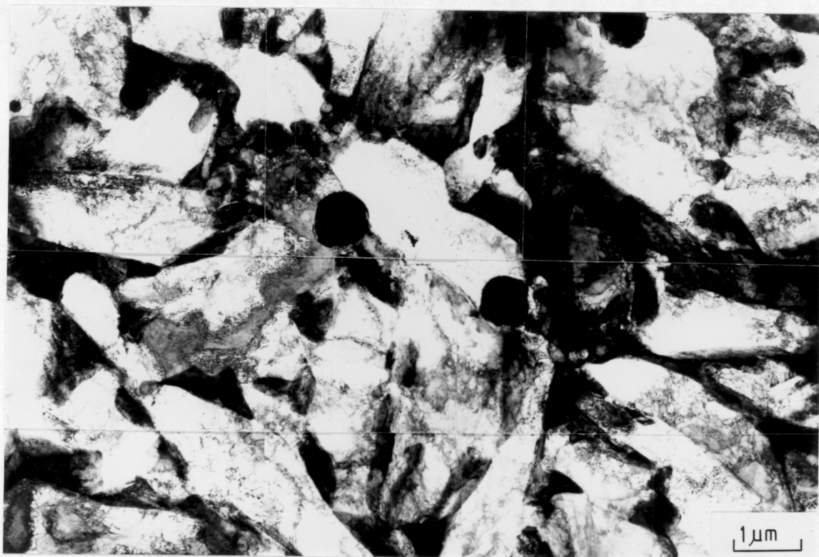
Figure IV.7(a) - Reaustenitisation at 680°C for 10 minutes from starting microstructure \alpha_a + \gamma .
