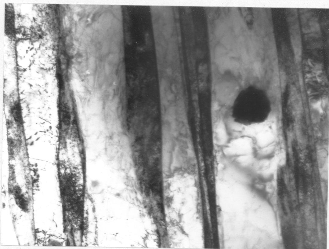
Figure IV.6(b) - Reaustenitisation at 700°C for 2 hours from starting microstructure \alpha_b + \gamma . 0.5 \mu m
