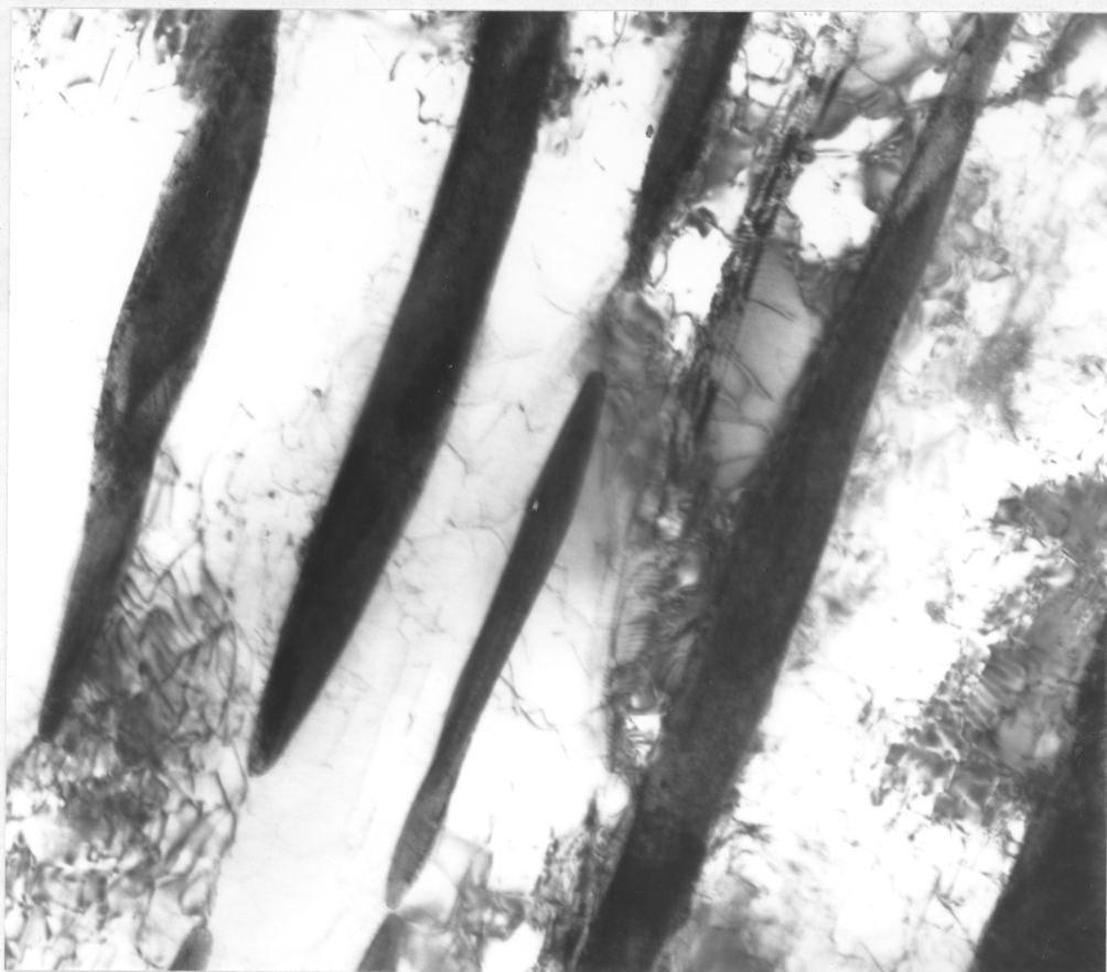
Figure IV.6(a) - Reaustenitisation at 680°C for 2 hours from starting microstructure \alpha_b + \gamma . 0.5 \mu m
