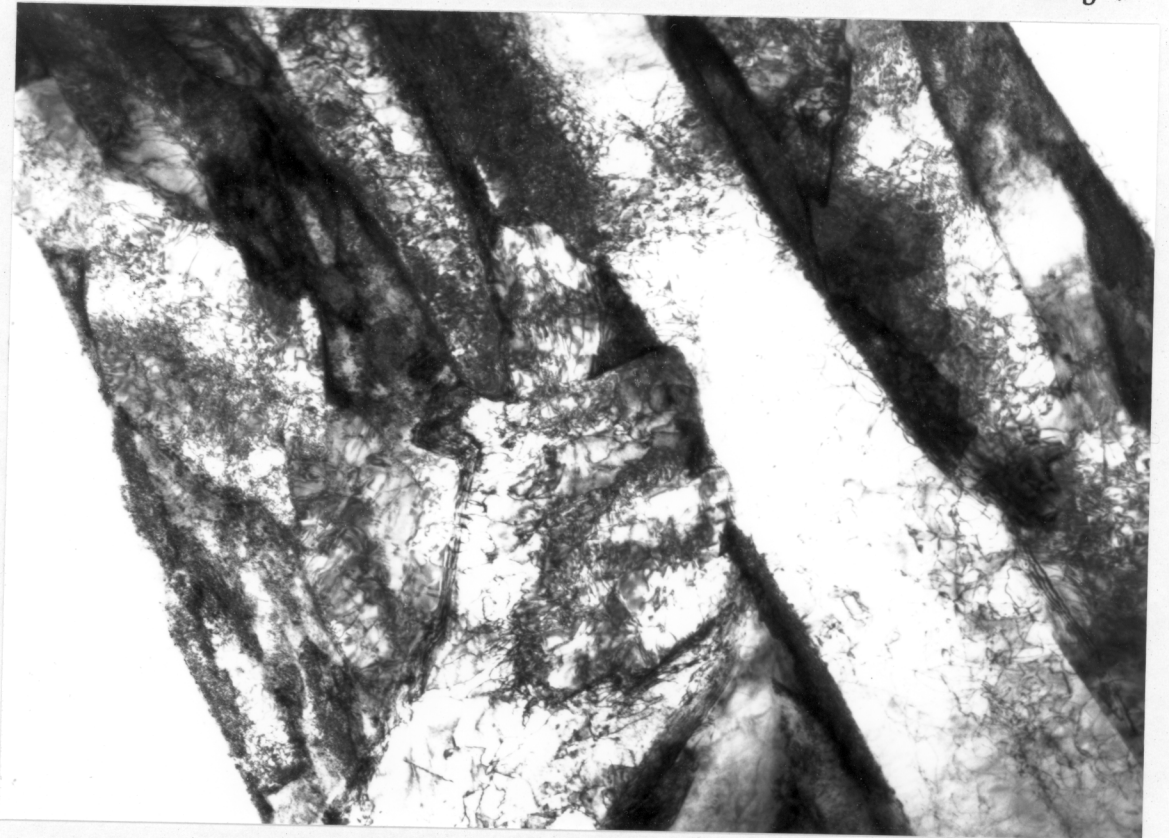
Figure IV.6(d) - Reaustenitisation at 740°C for 2 hours from starting microstructure \alpha_b + \gamma .
