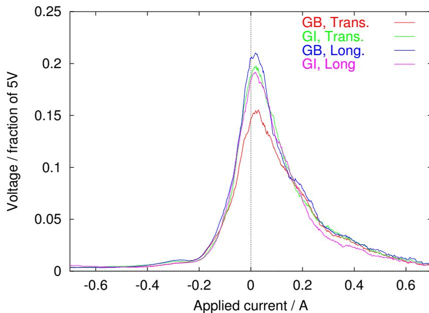
Figure 10.18: Effect on Barkhausen signal of magnetising across a grain boundary (GB) or grain interior (GI) in recrystallised PM2000.
