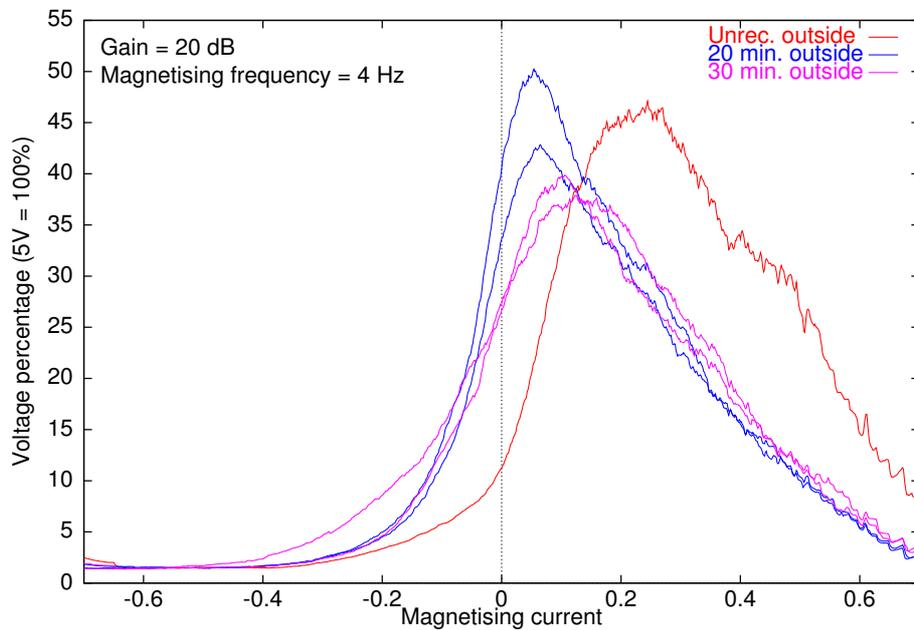
Figure 10.26: Barkhausen signal for outer surfaces of curved samples.
