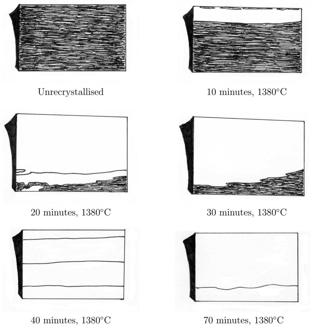
Figure 10.4: Sketches of microstructures of ODS material after different heat treatments. The tube axis is horizontal and the upper edge closer to the outer tube edge.
