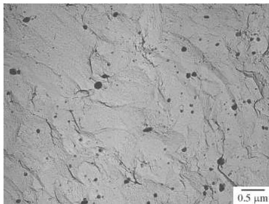
Figure 10.1: Oxide particles in PM2000 microstructure. Micrograph by C. Capdevila Montes; used with permission.
