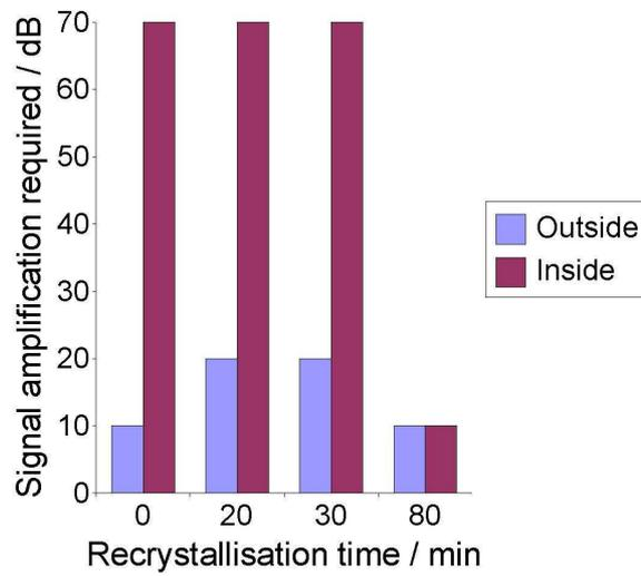
Figure 10.25: The amplifications needed for a visible signal from unprepared samples of PM2000.
