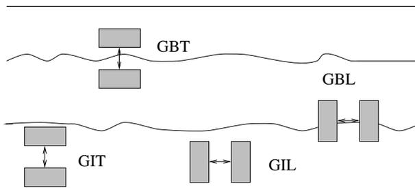
Figure 10.17: Positions in which Barkhausen signal was measured. GB, GI are grain boundary and grain interior; L and T are longitudinal and transverse.
