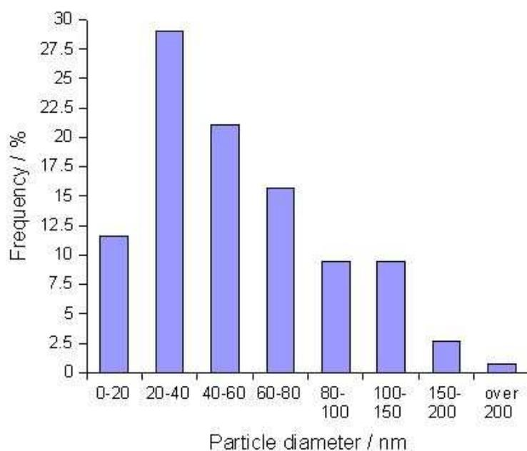
Figure 10.2: Oxide particle size distribution (Capdevila Montes, personal communication).
