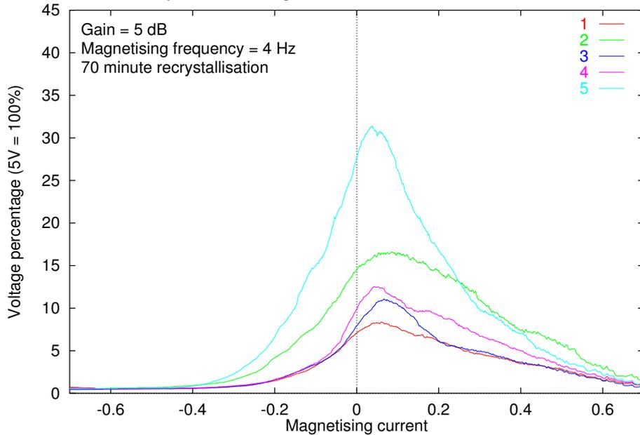
Figure 10.24: BN signals from samples heated at 1380°C for 70 minutes, measured in longitudinal direction. Lines 2 and 4 are signals measured along grain boundaries, and the others come from within the grains.
