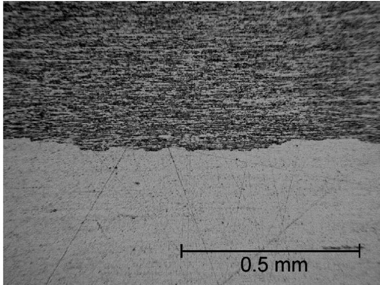
Figure 10.5: Optical micrograph showing recrystallised and unrecrystallised regions.
