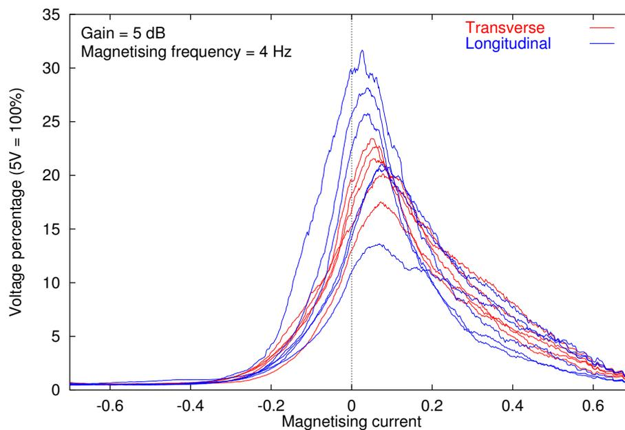
Figure 10.22: BN signals from samples heated at 1380°C for 20 minutes.
