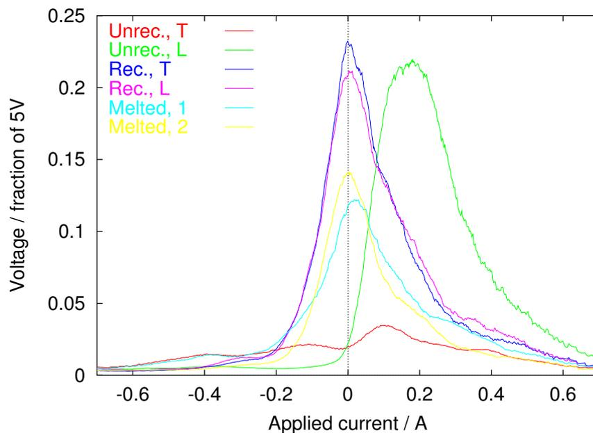
Figure 10.13: BN signals from unrecrystallised, recrystallised and melted PM2000 magnetised at 4 Hz.
