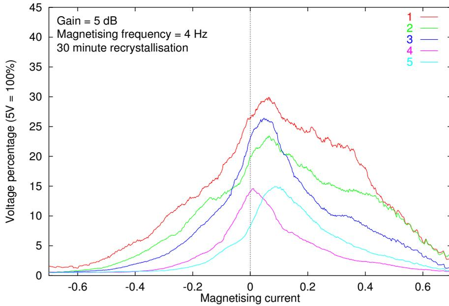
Figure 10.23: BN signals from samples heated at 1380°C for 30 minutes, measured in longitudinal direction. Line 4 was measured on the recrystallised/unrecrystallised boundary, line 5 in the unrecrystallised region, and the others in the recrystallised region.
