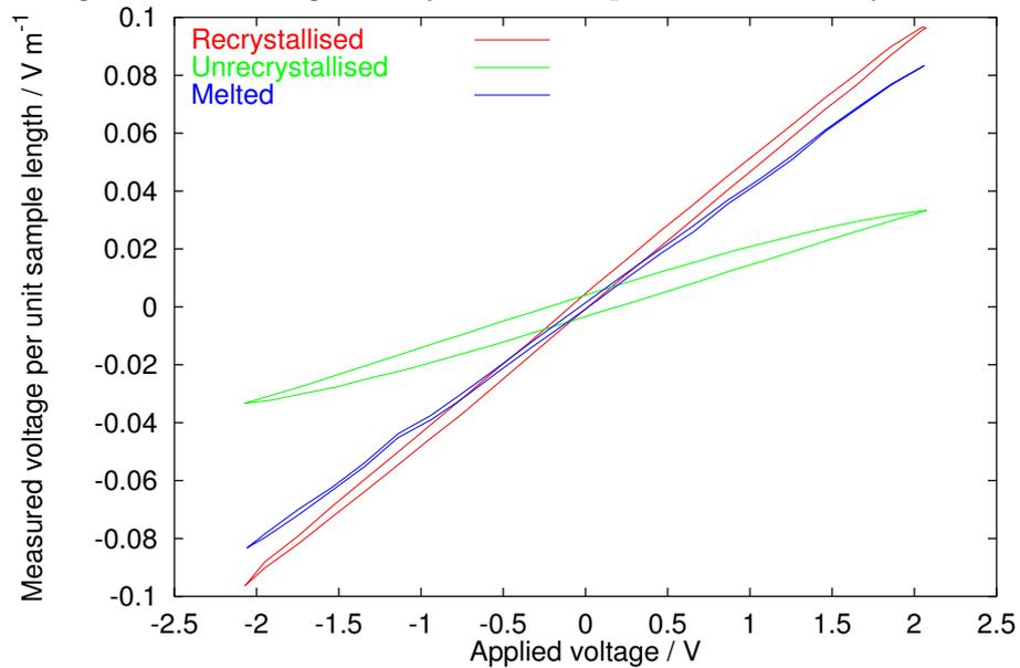
Figure 10.12: Magnetic hysteresis loops as measured by hysteresis unit.
