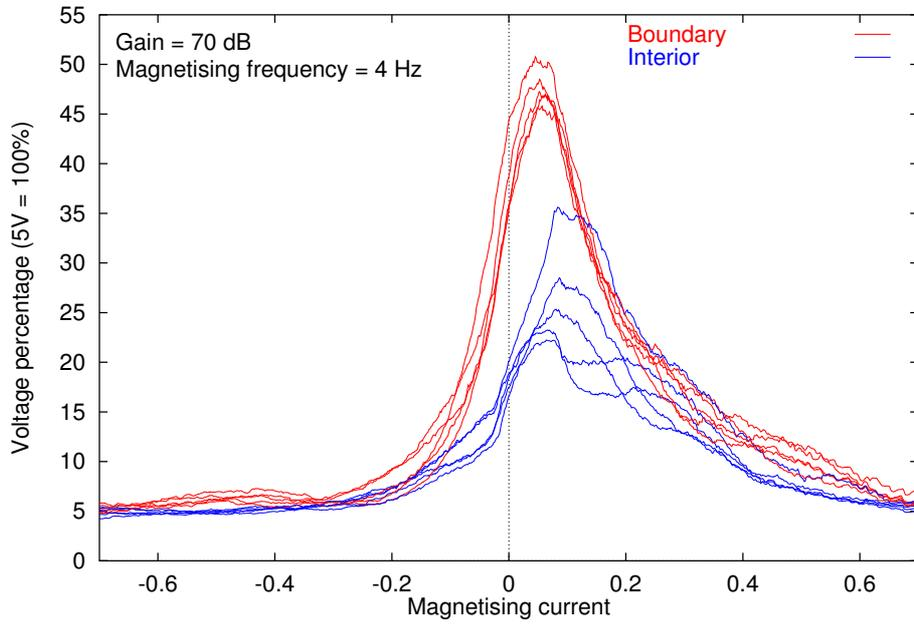
Figure 10.20: BN signals from samples heated at 1380°C for 10 minutes, measured perpendicular to tube length.
