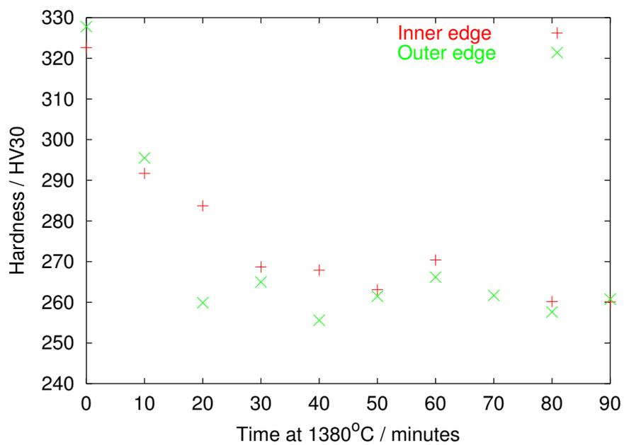
Figure 10.8: Hardness changes on heating PM2000 at 1380°C.
