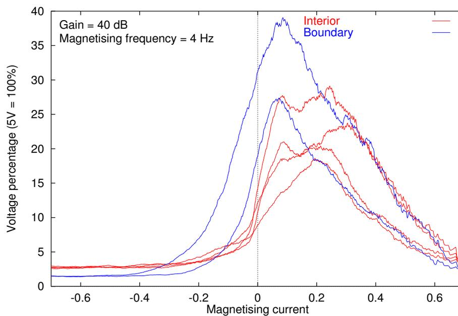
Figure 10.21: BN signals from samples heated at 1380°C for 10 minutes, measured parallel to tube length.
