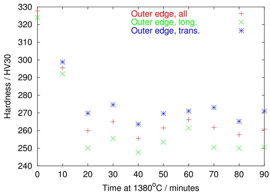
Figure 10.10: Hardness in longitudinal and transverse directions for outer edge.
