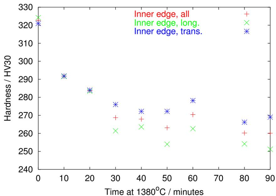
Figure 10.9: Hardness in longitudinal and transverse directions for inner edge.
