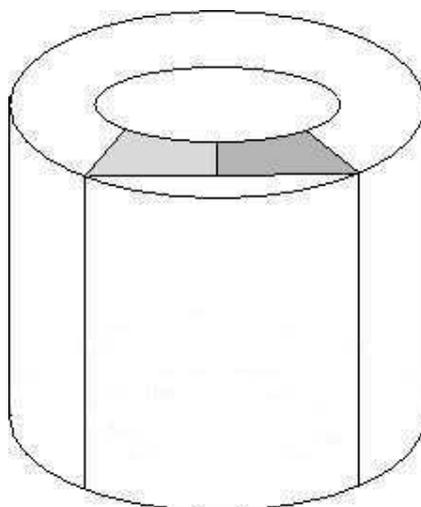
Figure 10.3: Origin of the tube-section samples, marked in grey.
