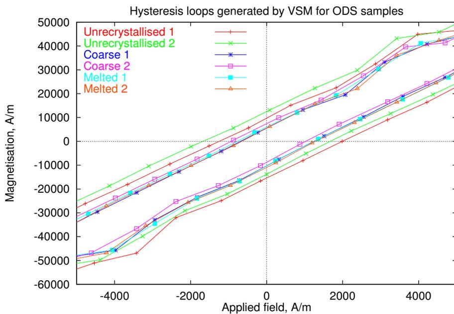
Figure 10.11: Magnetic hysteresis loops as measured by VSM.
