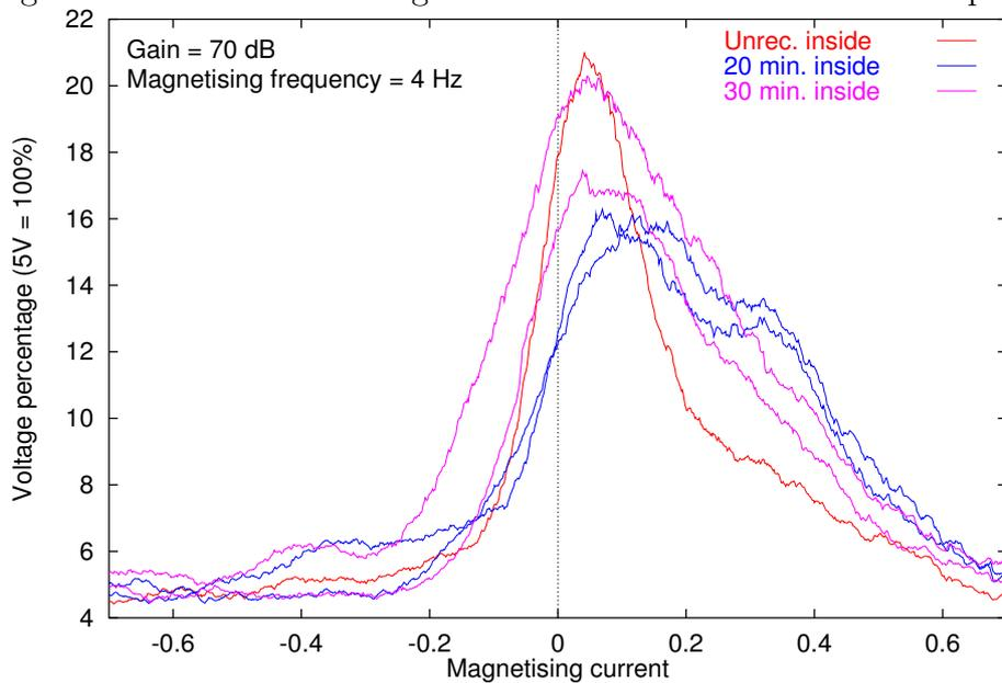
Figure 10.27: Barkhausen signal for inner surfaces of curved samples.
