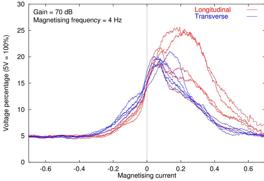
Figure 10.19: BN signal from unrecrystallised sample.
