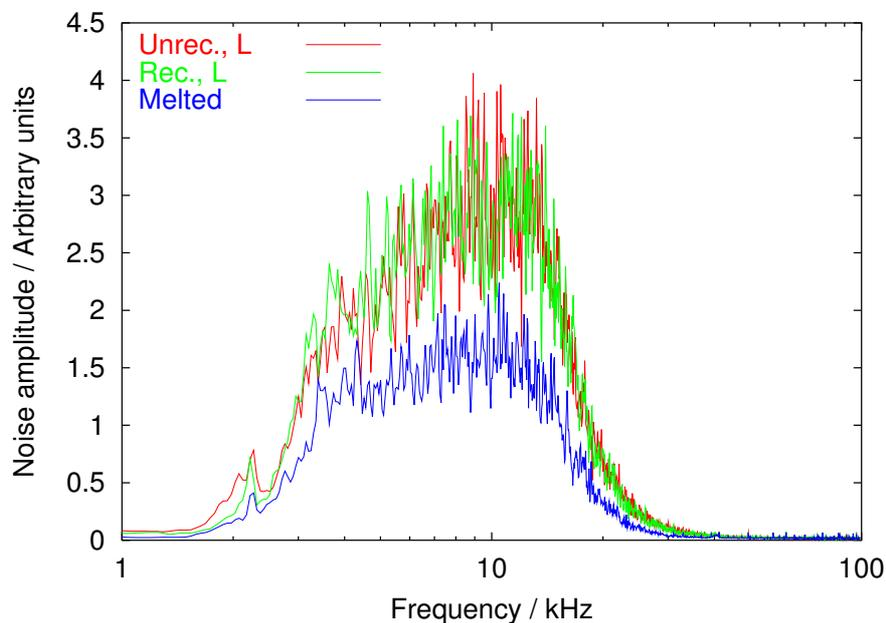
Figure 10.15: Frequency spectra from unrecrystallised, recrystallised and melted PM2000 magnetised at 4 Hz.
