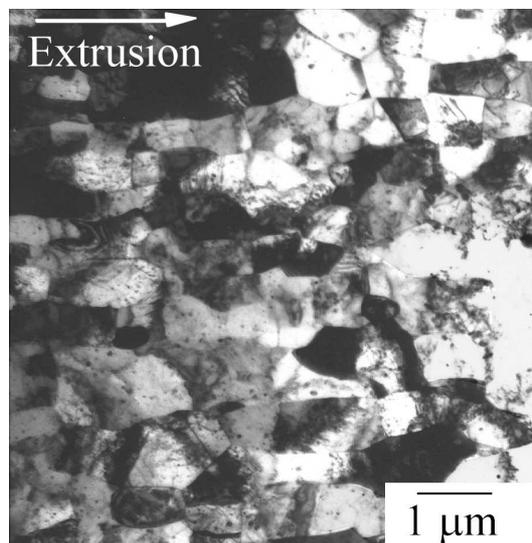
Figure 10.6: Unrecrystallised material observed using TEM. Micrograph by C. Capdevila Montes; used with permission.
