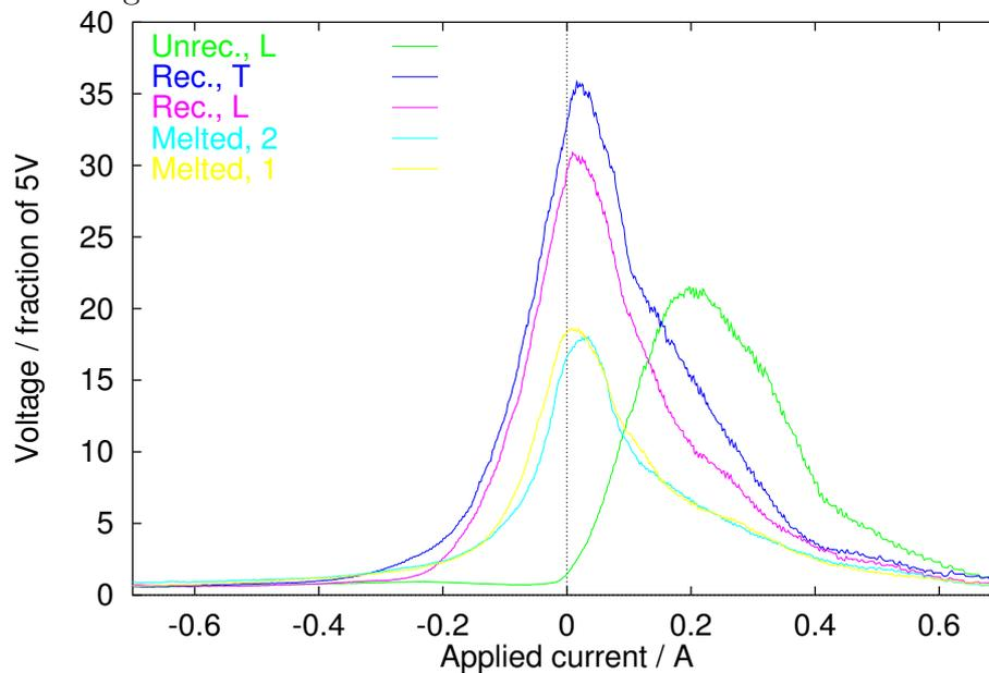
Figure 10.14: BN signals from unrecrystallised, recrystallised and melted PM2000 magnetised at 2 Hz.
