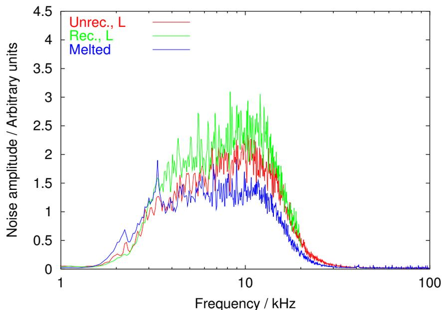
Figure 10.16: Frequency spectra from unrecrystallised, recrystallised and melted PM2000 magnetised at 2 Hz.
