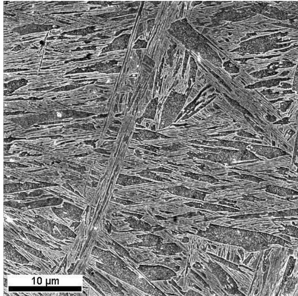
Figure 6.20: SEM micrograph of as-quenched  $2\frac{1}{4}$ Cr1Mo steel.
