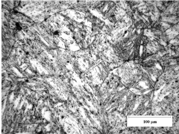
Figure 6.6:  $2\frac{1}{4}$ Cr1Mo steel tempered for 32 hours at 500°C.
