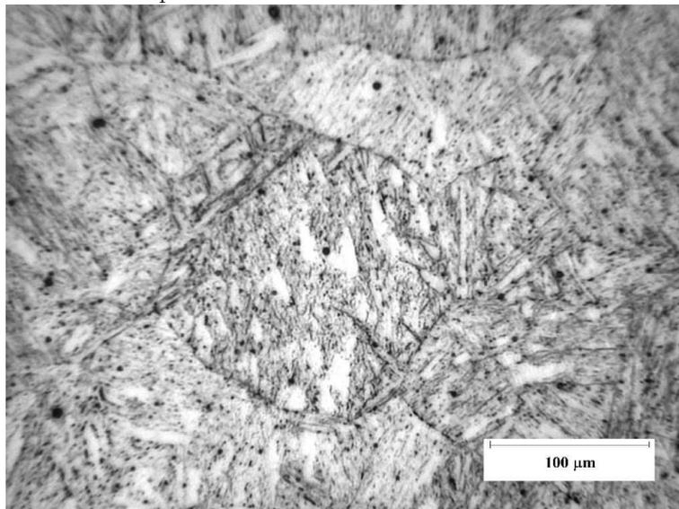
Figure 6.5:  $2\frac{1}{4}$ Cr1Mo steel tempered for 4 hours at 500°C.
