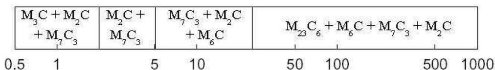
Figure 6.29: Carbide phase stability at 700°C in  $2\frac{1}{4}\text{Cr1Mo}$  steel, after Nutting (1998).
