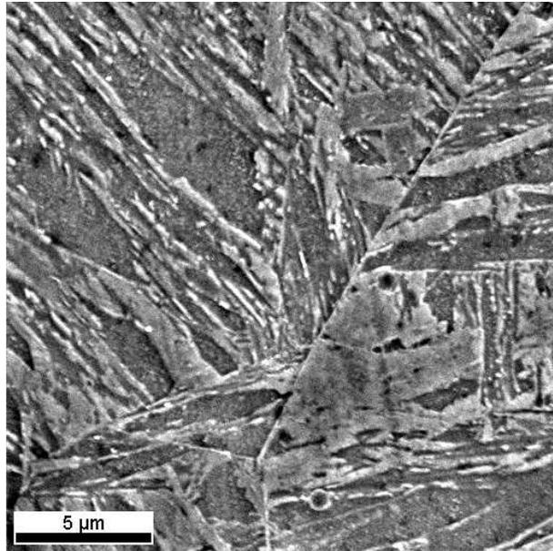
Figure 6.22: SEM micrograph of  $2\frac{1}{4}\text{Cr1Mo}$  steel tempered at  $500^\circ\text{C}$  for 1 hour.
