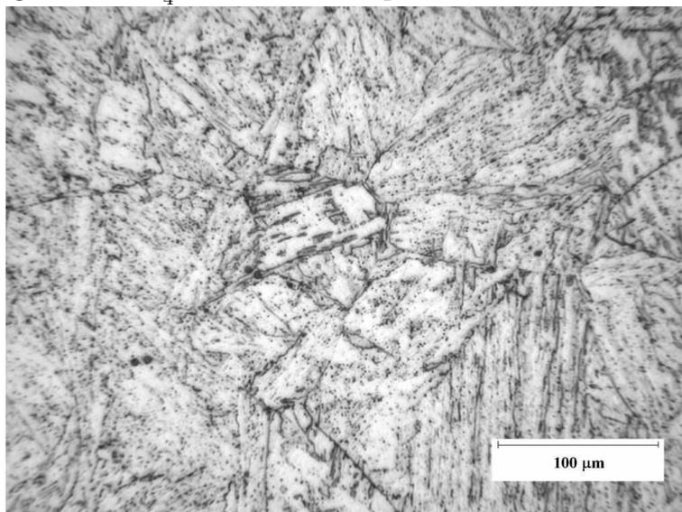
Figure 6.13:  $2\frac{1}{4}$ Cr1Mo steel tempered for 2 hours at 700°C.
