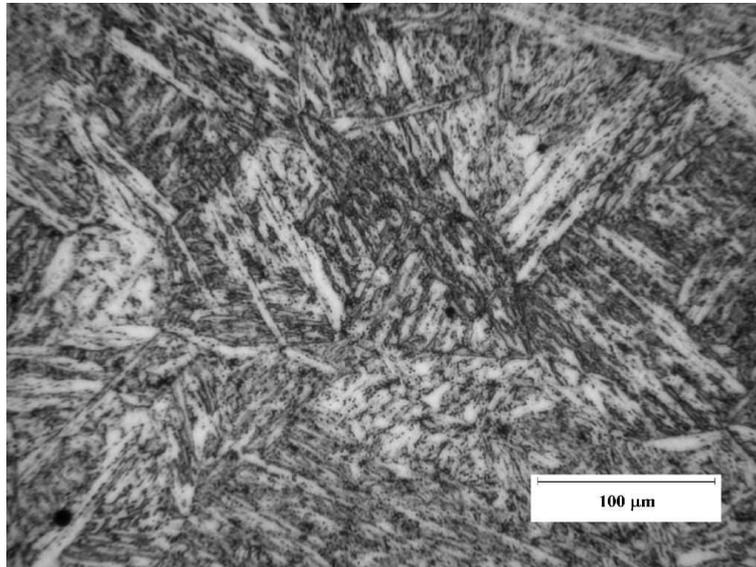
Figure 6.16: 11 wt. % Cr steel heated for 2347 hours at 550°C during creep test.
