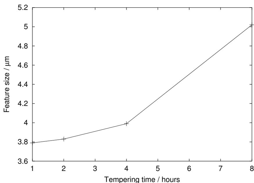
Figure 6.27: Changes in average feature spacing with tempering time at 700°C.
