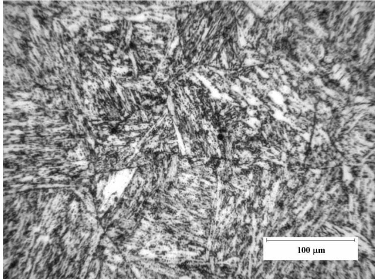
Figure 6.18: 11 wt. % Cr steel heated for 16530 hours at 550°C during creep test.
