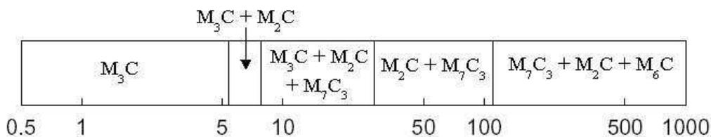
Figure 6.28: Carbide phase stability at 600°C in  $2\frac{1}{4}\text{Cr1Mo}$  steel, after Nutting (1998).
