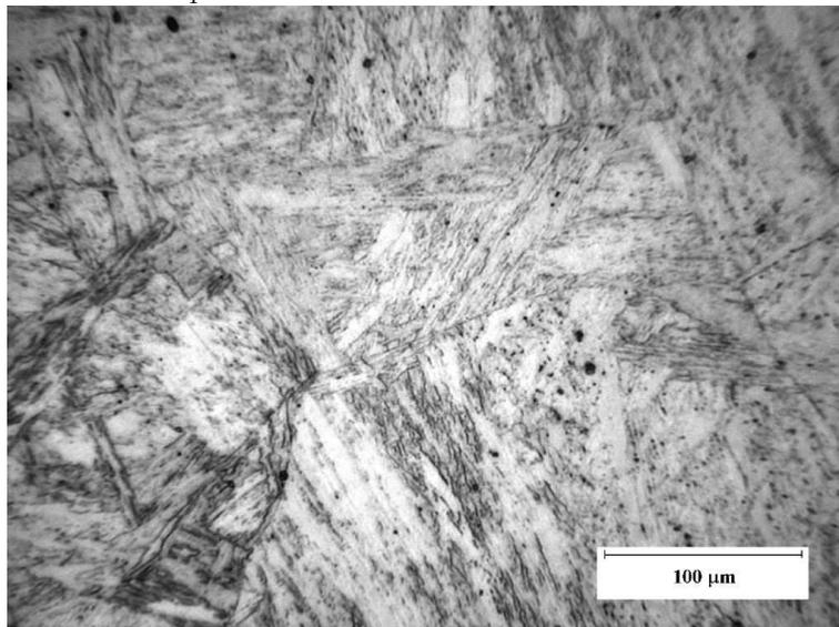
Figure 6.9:  $2\frac{1}{4}$ Cr1Mo steel tempered for 16 hours at 600°C.
