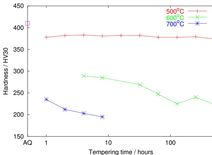
Figure 6.30: Hardness of tempered  $2\frac{1}{4}$ Cr1Mo steel samples.
