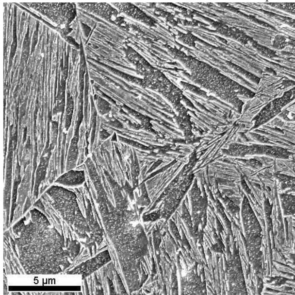
Figure 6.21: SEM micrograph of as-quenched  $2\frac{1}{4}$ Cr1Mo steel.
