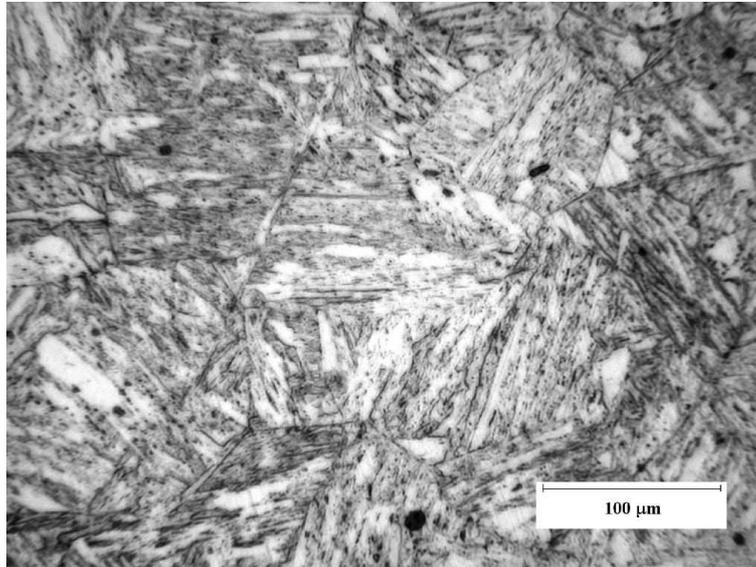
Figure 6.4:  $2\frac{1}{4}$ Cr1Mo steel tempered for 1 hour at 500°C.
