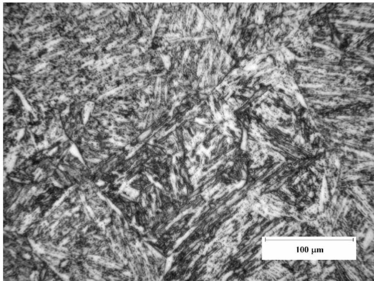
Figure 6.17: 11 wt. % Cr steel heated for 5849 hours at 550°C during creep test.
