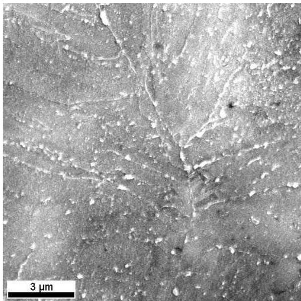
Figure 6.26: SEM micrograph of  $2\frac{1}{4}\text{Cr1Mo}$  steel tempered at  $700^\circ\text{C}$  for 1 hour.
