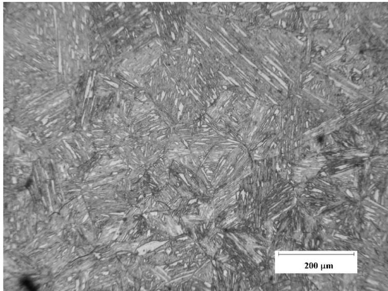
Figure 6.2: As-quenched microstructure of  $2\frac{1}{4}$ Cr1Mo steel.
