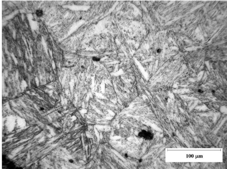
Figure 6.8:  $2\frac{1}{4}$ Cr1Mo steel tempered for 4 hours at 600°C.
