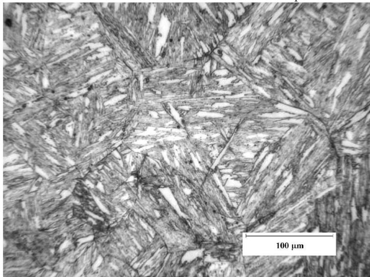
Figure 6.3: As-quenched microstructure of  $2\frac{1}{4}$ Cr1Mo steel.
