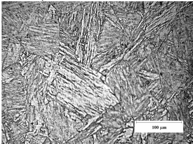
Figure 6.11:  $2\frac{1}{4}$ Cr1Mo steel tempered for 512 hours at 600°C.
