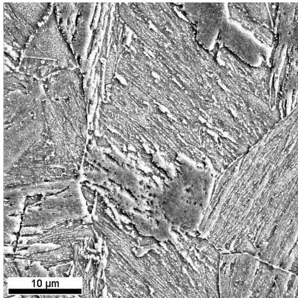
Figure 6.25: SEM micrograph of  $2\frac{1}{4}$ Cr1Mo steel tempered at 600°C for 256 hours.
