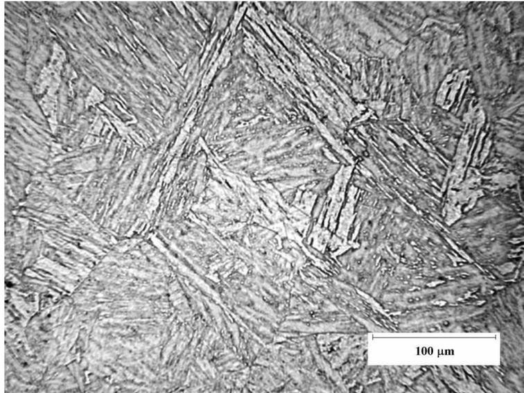
Figure 6.10:  $2\frac{1}{4}$ Cr1Mo steel tempered for 256 hours at 600°C.
