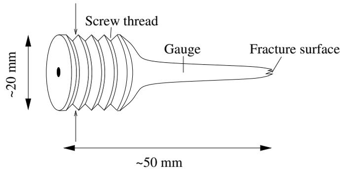
Figure 6.1: Failed creep test specimen. The arrows show the position at which the Barkhausen test specimen was cut.
