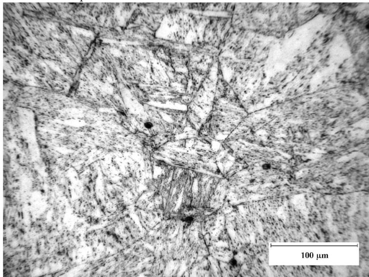
Figure 6.7:  $2\frac{1}{4}$ Cr1Mo steel tempered for 256 hours at 500°C.
