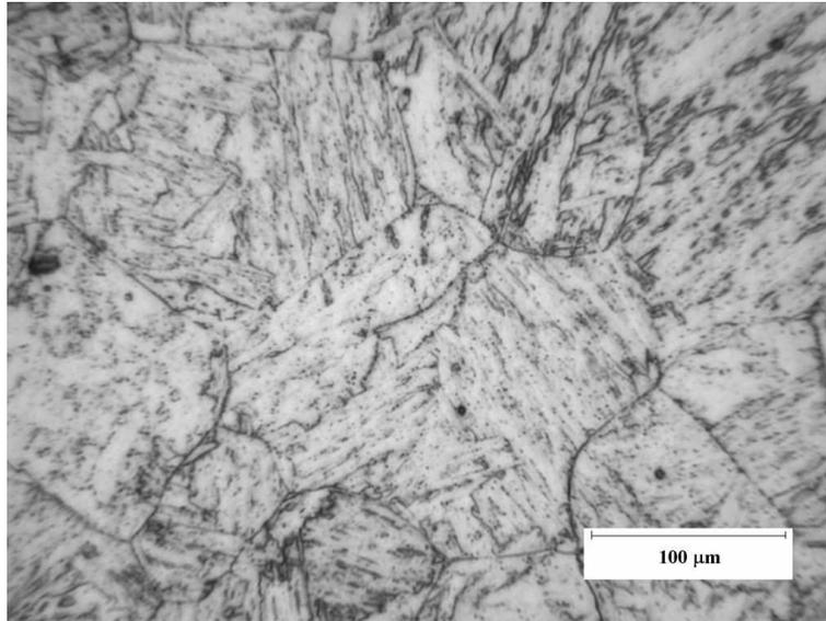
Figure 6.14:  $2\frac{1}{4}$ Cr1Mo steel tempered for 4 hours at 700°C.
