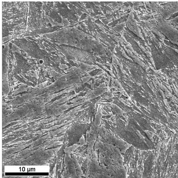
Figure 6.23: SEM micrograph of  $2\frac{1}{4}\text{Cr1Mo}$  steel tempered at  $500^\circ\text{C}$  for 256 hours.
