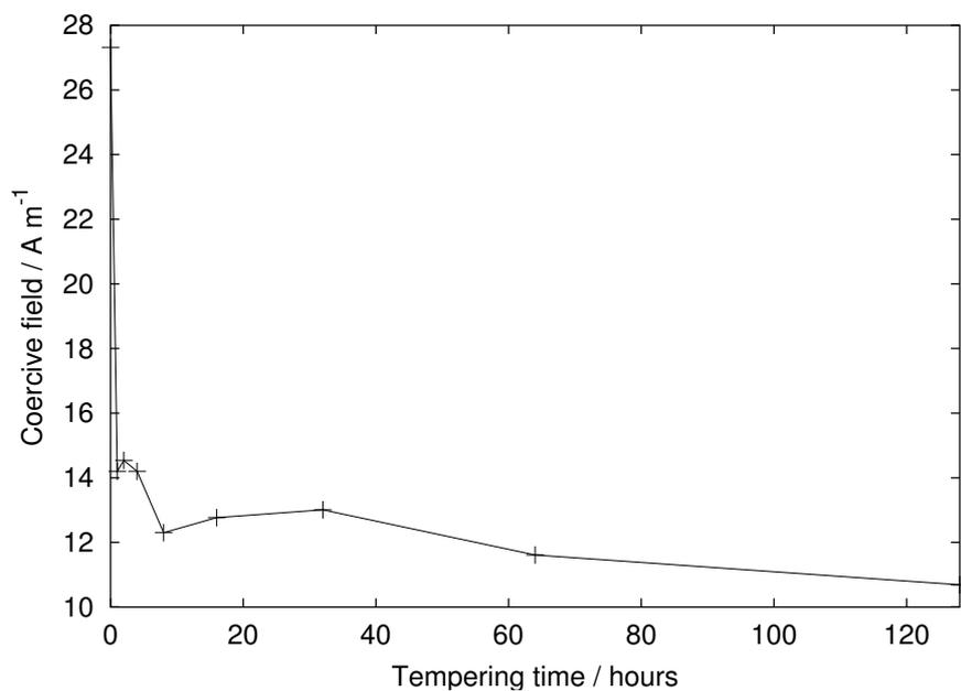
Figure 6.32: Coercive field of 2 $\frac{1}{4}$ Cr1Mo steel tempered at 600°C. Data from M.Sci. dissertation of present author, 1999.
