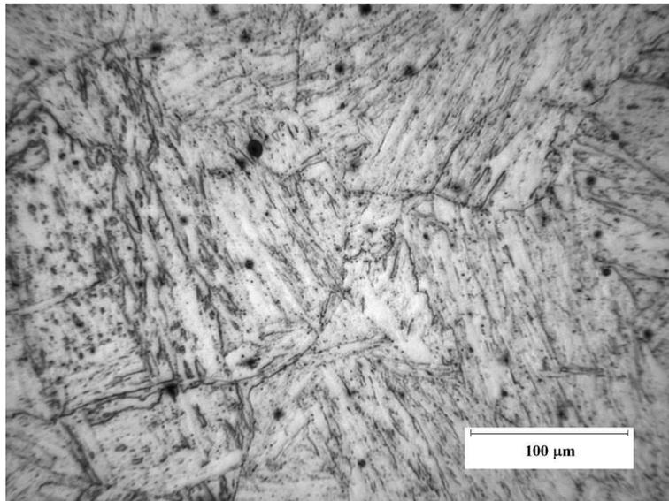
Figure 6.12:  $2\frac{1}{4}$ Cr1Mo steel tempered for 1 hour at 700°C.
