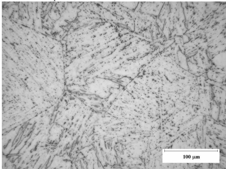
Figure 6.15:  $2\frac{1}{4}$ Cr1Mo steel tempered for 8 hours at 700°C.
