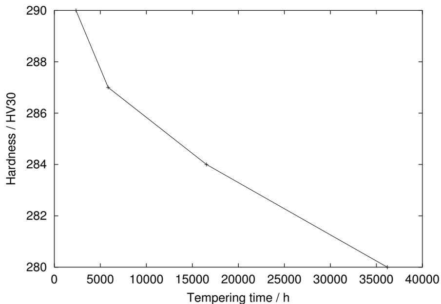
Figure 6.31: Hardness of creep-tested 11Cr1Mo wt. % steel samples.
