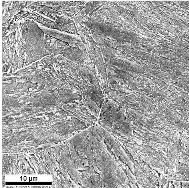
Figure 6.24: SEM micrograph of  $2\frac{1}{4}$ Cr1Mo steel tempered at 600°C for 16 hours.
