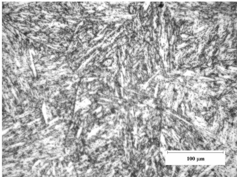
Figure 6.19: 11 wt. % Cr steel heated for 36191 hours at 550°C during creep test.
