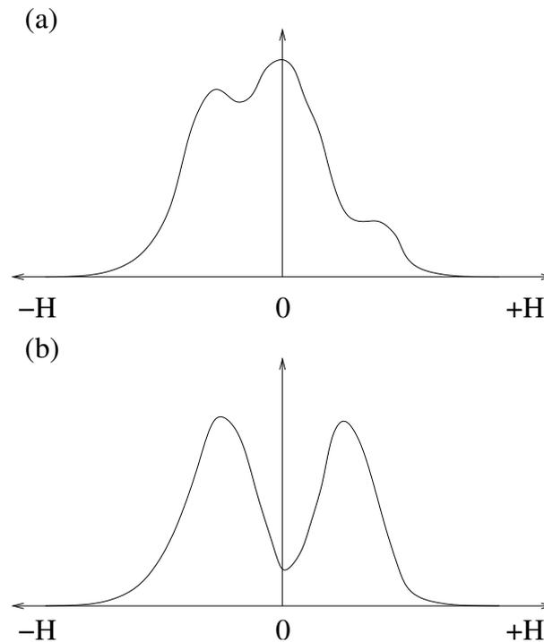
Figure 4.7: (a) BN signal from pure iron, cold-worked and annealed below 550°C; (b) MAE signal from the same sample (Buttle *et al.*, 1987a).
