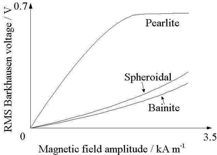
Figure 4.19: Dependence of the RMS BN voltage on applied field amplitude, after Mitra *et al.*, 1995
