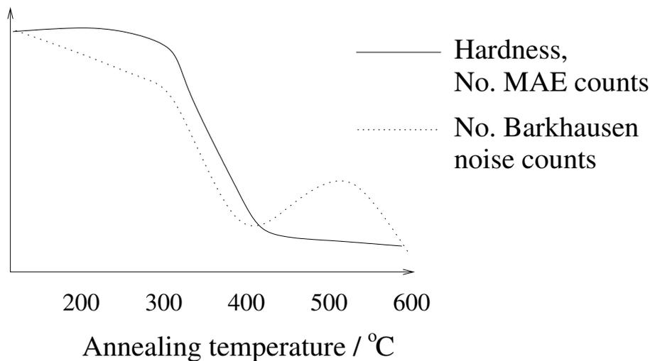
Figure 4.6: Effect of annealing temperature on mechanical and magnetic properties of deformed nickel (Ranjan *et al.*, 1987c).
