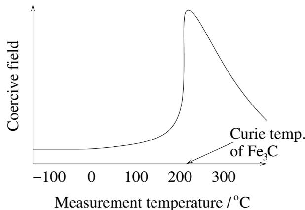
Figure 4.9: Anomaly in the coercive field predicted at the Curie temperature of  $\text{Fe}_3\text{C}$  (English, 1967).
