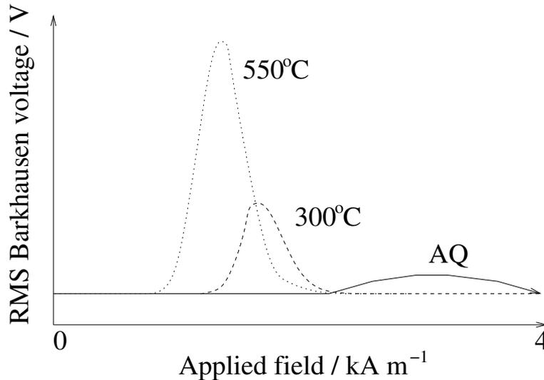
Figure 4.15: Change in the shape of the BN signal from as-quenched (AQ) state due to tempering for one hour at 300 and 550°C (Saquet *et al.*, 1999).
