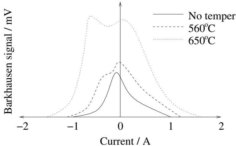
Figure 4.14: Changes in BN peak size and shape due to tempering (Buttle *et al.*, 1987c).
