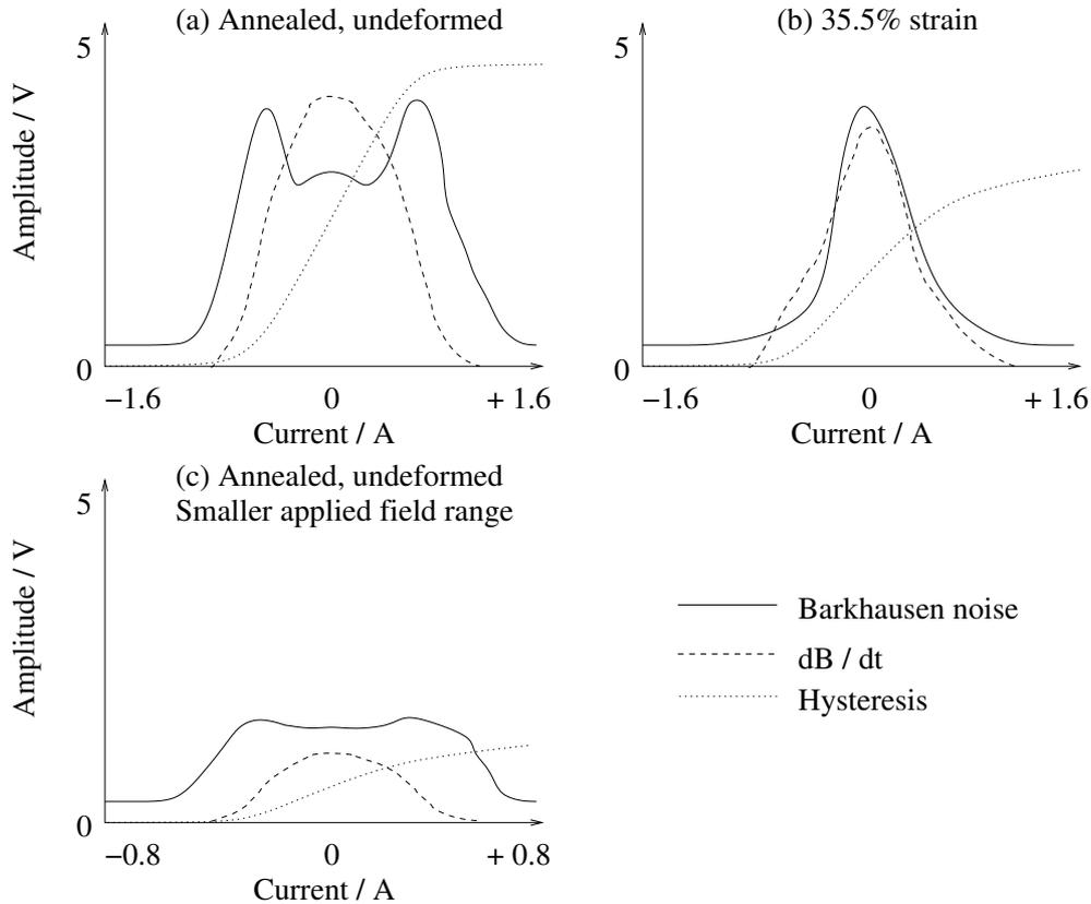
Figure 4.8: Effect of straining and changing the applied current range (and hence  $H_{\max}$ ) on BN, hysteresis and  $dB/dt$  curves (Kim *et al.*, 1992).
