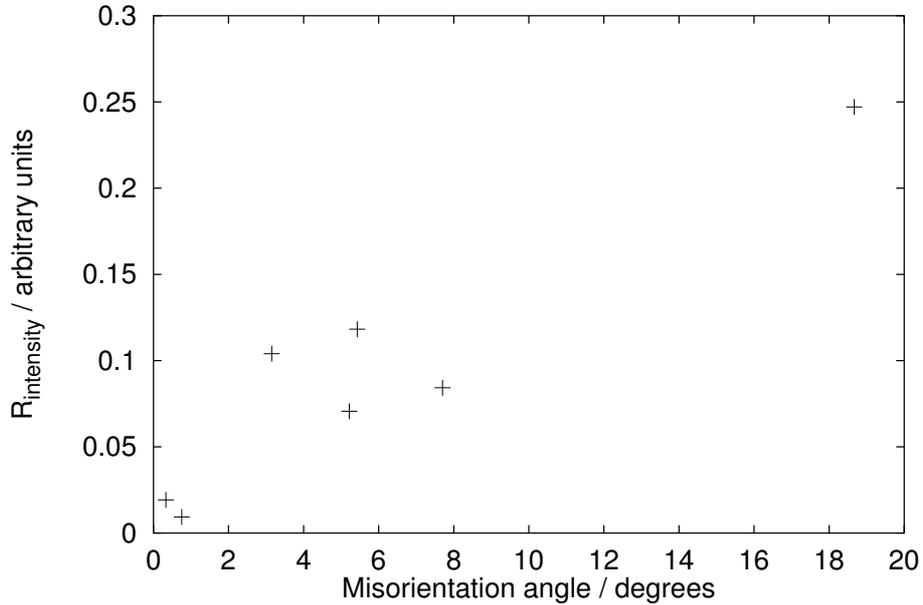
Figure 4.4: Dependence of  $R_{\text{intensity}}$  on misorientation angle in Fe-3 wt. % Si (Yamaura *et al.*, 2001).
