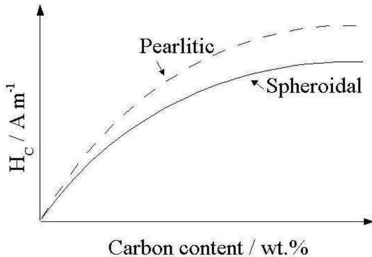
Figure 4.10: The effect of carbon content on coercive field in plain-carbon steel, for spheroidal and pearlitic microstructures (Jiles, 1988a).
