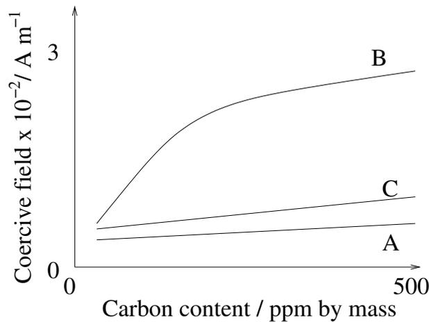
Figure 4.11: The effects of different precipitation states on the coercive field (A) carbon mostly in interstitial solution, (B) intragranular precipitates of around  $0.5 \mu\text{m}$  diameter, (C) large carbides of around  $10 \mu\text{m}$  diameter at grain boundaries (Lopez *et al.*, 1985).
