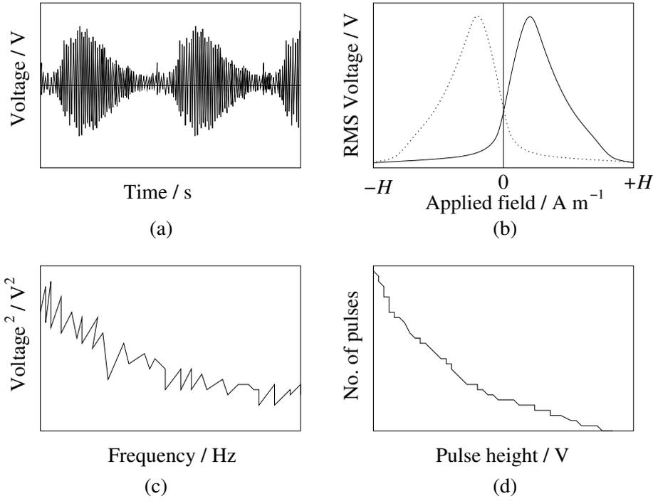
Figure 4.3: Magnetic noise plots: (a) Raw noise versus time. (b) Root-mean-square (RMS) noise versus applied field. (c) Noise voltage versus frequency (Fourier transform). (d) Pulse height distribution plot.
