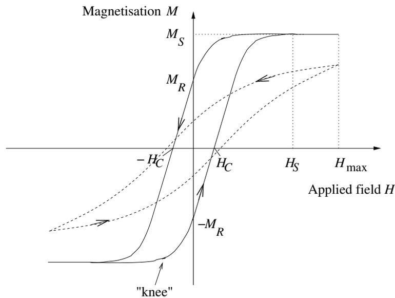
Figure 4.1: A major hysteresis loop (solid line), showing the coercive field  $H_C$ , remanence  $M_R$  and saturation magnetisation  $M_S$ , and a minor loop (dashed line). The arrows show the direction of magnetisation.
