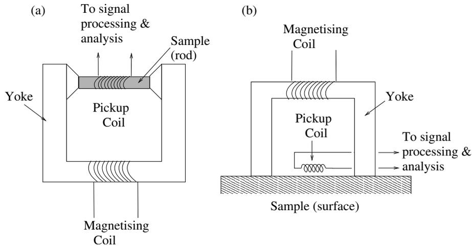
Figure 4.2: Typical measurement apparatus for magnetic noise: (a) magnetising yoke with rod-shaped specimen, (b) surface sensor.
