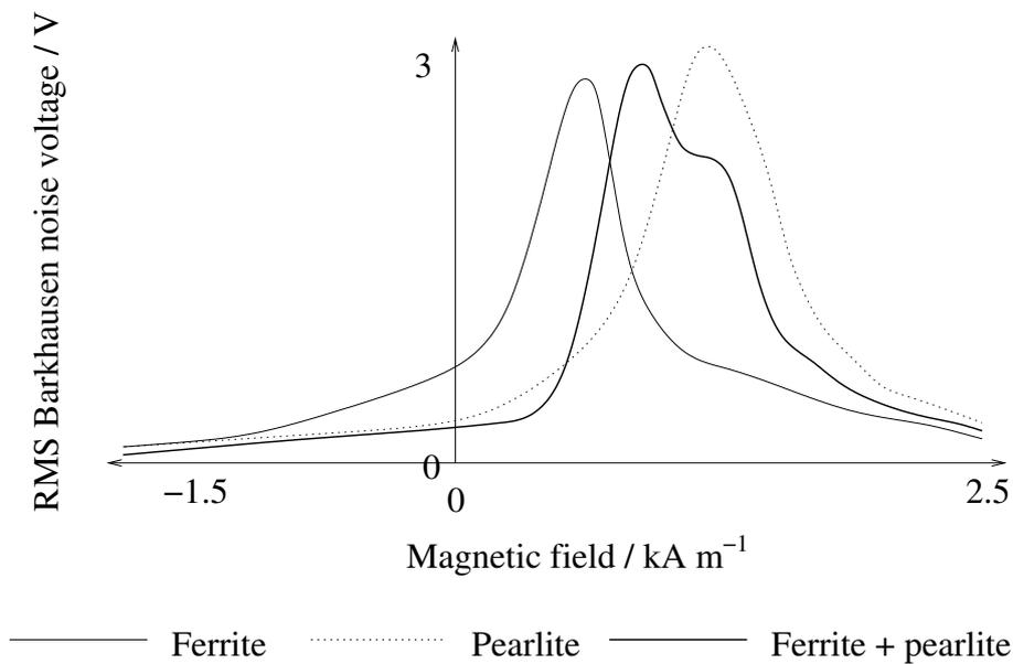
Figure 4.12: BN signals from ferritic, pearlitic and ferrite + pearlite microstructures in plain-carbon steel, showing two-component signal from the microstructure with two constituents (Saquet *et al.*, 1999).
