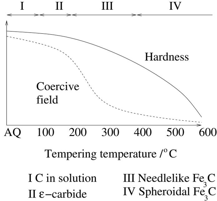
Figure 4.13: Changes in hardness and coercive field associated with different tempering times (Kameda and Ranjan, 1987a).
