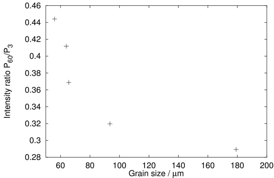
Figure 4.5: Relationship between frequency components of BN and grain size (Yamaura *et al.*, 2001).
