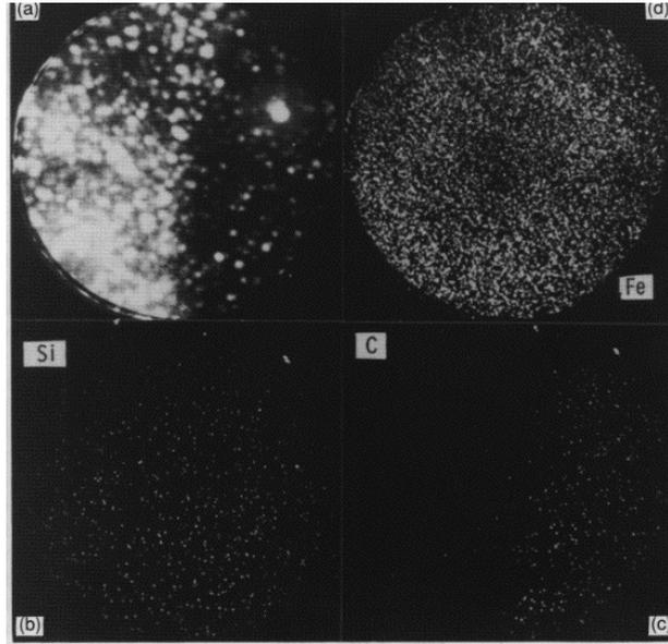
Fig. 7: Imaging atom-probe micrographs, taken across an austenite-bainitic ferrite interface in a Fe-C-Si-Mn alloy. The images confirm quantitative data (Bhadeshia and Waugh, 1982) showing the absence of any substitutional atom diffusion during transformation. (a) Field-ion image; (b) corresponding silicon map; (c) corresponding carbon map; (d) corresponding iron map.
