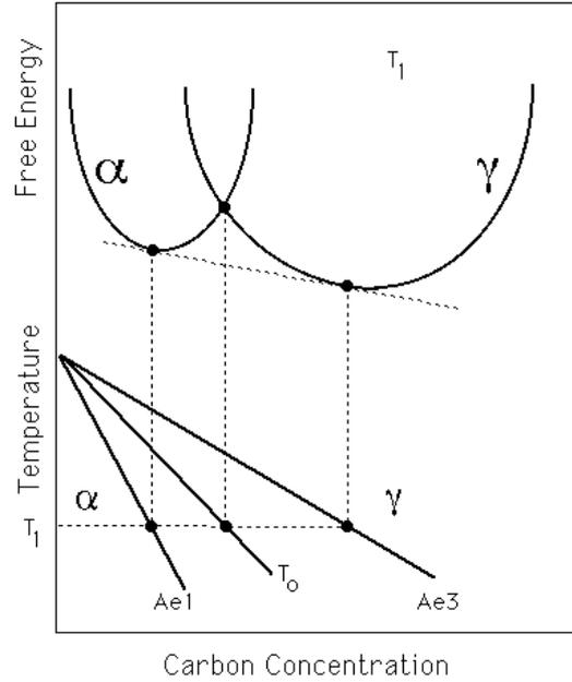
Fig. 8: Schematic illustration of the origin of the  $T_0$  construction on the Fe–C phase diagram. Austenite with a carbon concentration to the left of the  $T_0$  boundary can in principle transform without any diffusion. Diffusionless transformation is thermodynamically impossible if the carbon concentration of the austenite exceeds the  $T_0$  curve.
