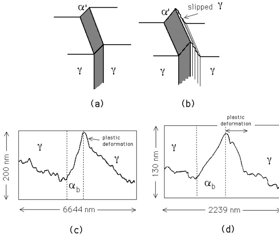
Fig. 6: (a) A perfect invariant–plane strain surface relief effect. (b) One where plastic relaxation of the shape change occurs in the adjacent matrix. (c,d) An actual atomic force microscope scan across the surface relief due to a bainite sub–unit (Swallow and Bhadeshia, 1996).
